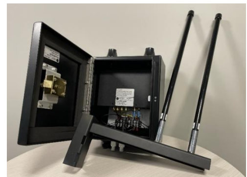
RSU (cabinet hardware with antenna)
